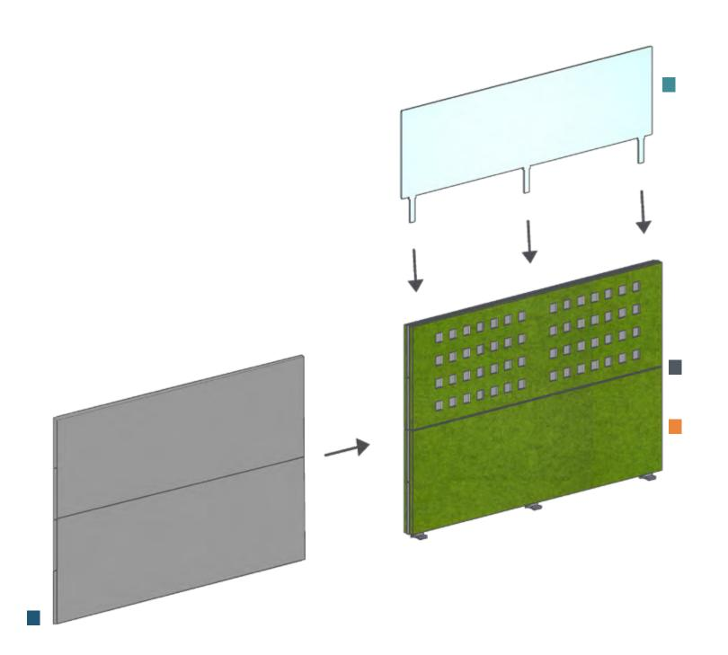
**Blocking** For added sound control, WHISPER allows for a vinyl sound-blocking insert when more privacy is needed. Sound-blocking insert further provides a lovely three-dimensional effect when used with perforated options.
